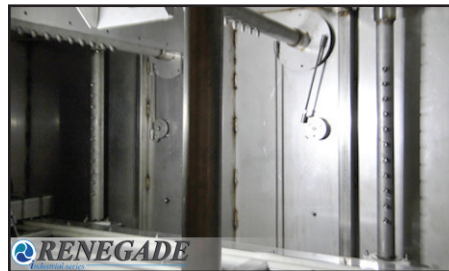
Oscillating spray manifolds and blower manifolds positioned for upper, lower, and side direction deliver high volume force for maximum cleaning and drying. Rugged variable-speed conveyor system with custom fixture carts.
