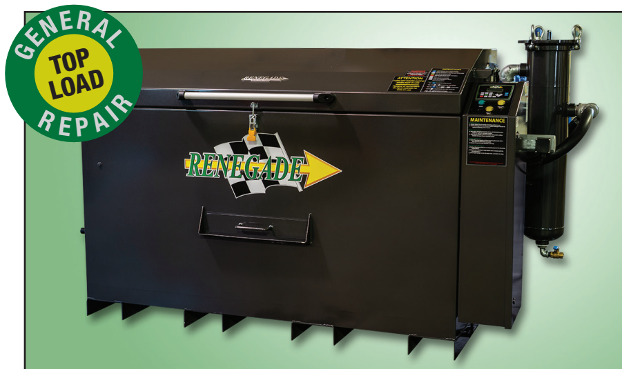
TMB 8100 STRETCH HRPW Dimensions Height: 50½ inches; Width: 90¼ inches; Depth: 58 inches Model above shown with Sump Sweep and Filtration Option
