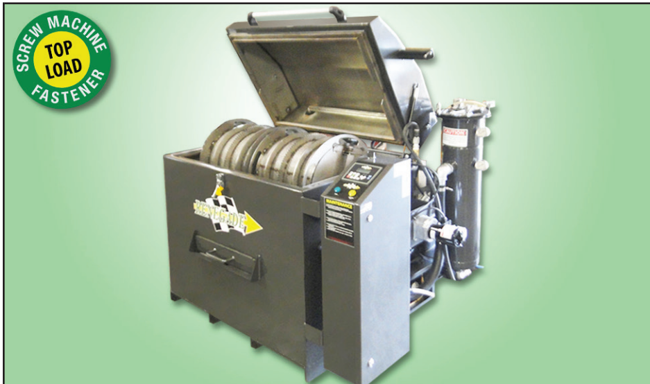
TLT Dual 1615 Tumbler Dimensions: Height: 49-1/4" inches; Width: 58-1/2" inches; Depth: 57" inches
