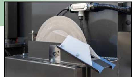
Oil Skimmer and Low Water Safety
